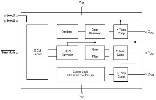
Figure 2. Simplified Accelerometer Functional Block Diagram
