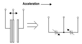
Figure 3. Simplified Transducer Physical Model
