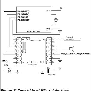
Figure 3: Typical Host Micro Interface
