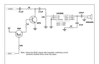
Figure 1: Optional Power Audio Circuit
