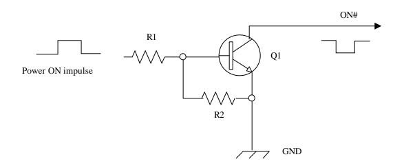
**NOTE:** don't use any pull up resistor on the ON# line, it is internally pulled up. Using pull up resistor may bring to latch up problems on the GM862-GPRS power regulator and improper power on/off of the module. The line ON# must be connected only in open collector configuration.
