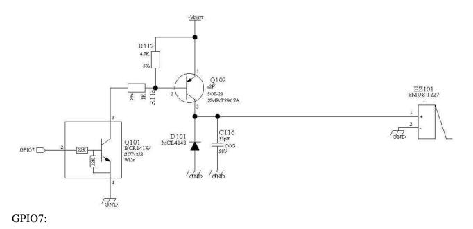
NOTE: To correctly drive a buzzer a driver must be provided, its characteristics depend on the Buzzer and for them refer to your buzzer vendor.
