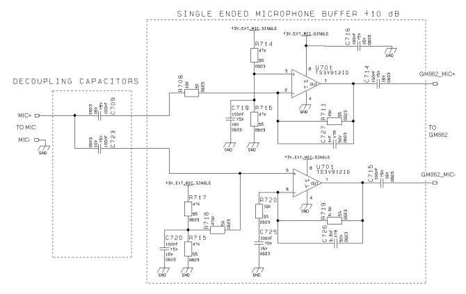
The schematic does not include the required mic. biasing circuitry. For the biasing the same circuit as seen before can be used; to be noticed that the capacitor C3 on the unbalanced biasing circuit is not anymore needed if this Buffered design is used.
