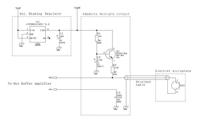
**NOTE:** In the unbalanced application the capacitor C3 shall be > 200nF otherwise the frequency response will be cut at low band frequencies (down to 300Hz). This capacitor can be placed close to the MIC- pin (EXT\_MIC- or INT\_MIC- depending on the audio path chosen) or if possible it should be placed close to the shielded cable connector. If the ground return path is well designed, then it is possible to eliminate the C3 capacitor, provided the buffer is close to the mic. input.
