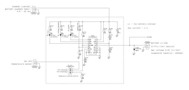
NOTE: In this particular application the battery charger input current must be limited to less than 1A. This can be done by using a current limited wall adapter as the power source.
