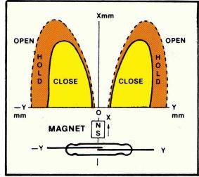
Figure 4 – Magnet Perpendicular to Reed Sw.
