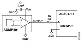
Figure 9. ADMP401 Connected to the ADAU1761 Codec
