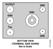
Figure 3. Pin Configuration (Bottom View)
