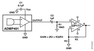
Figure 10. ADMP401 Connected to the OP177 Op Amp
