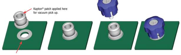
Solder paste applied to pad on PCB.
