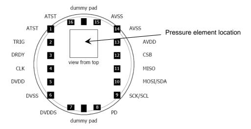
Figure 1 Pin arrangement of SCP1000
