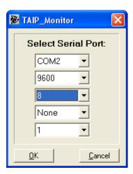
Figure E.1 TAIP Monitor - Serial Port Selection
