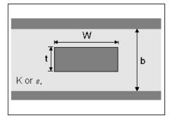
Figure 6.3 Stripline Transmission Lines
