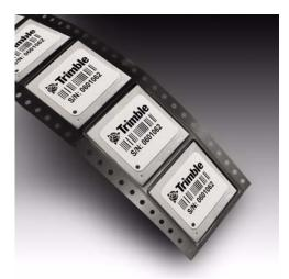
Figure 8.1 Copernicus GPS Receiver Packaged in Tape
