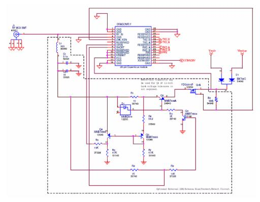
Figure 5.3 Application Drawing: Active antenna - Full connection
