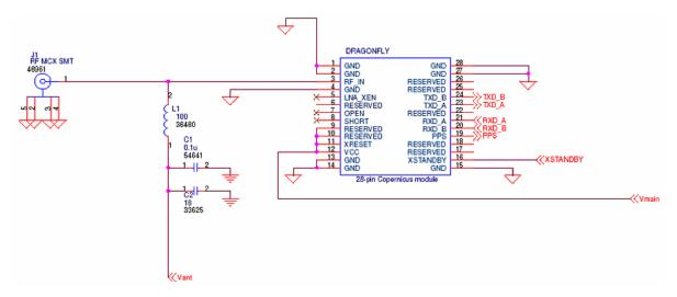
Figure 5.4 Application Drawing: Active antenna - No Antenna Status
