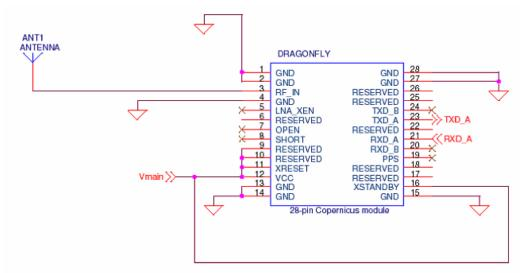
Figure 5.1 Application Drawing: Passive Antenna - Minimum Connections
