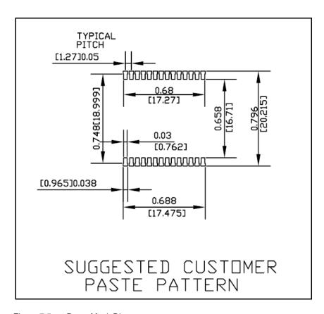
Figure 7.5 Paste Mask Diagram
