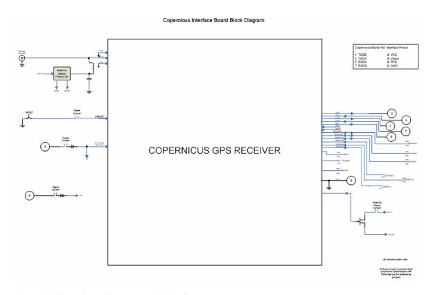
Figure 10.3 Copernicus Reference Board Block Diagram
