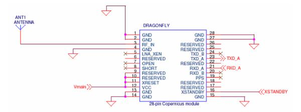
Figure 5.2 Passive antenna - HW Activated Standby Mode Available
