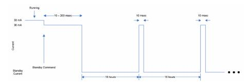
Figure 4.1 Current Draw Levels in Standby Mode
