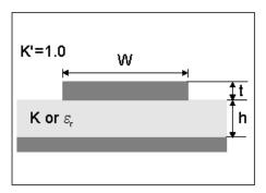
Figure 6.1 Microstrip Transmission Lines
