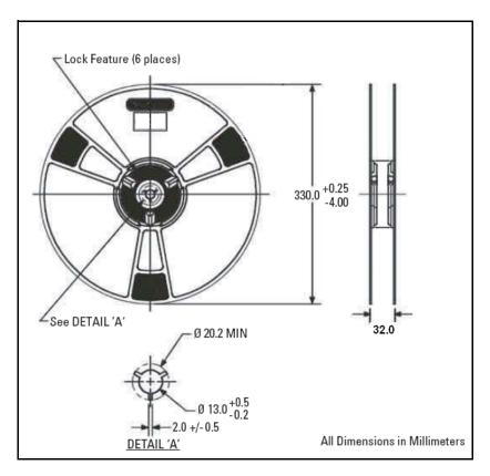
Figure 8.2 Reel Diagram
