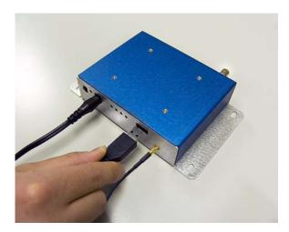
Figure 11.7 Connecting the Antenna
