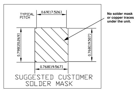
Figure 7.3 Solder Mask Diagram
