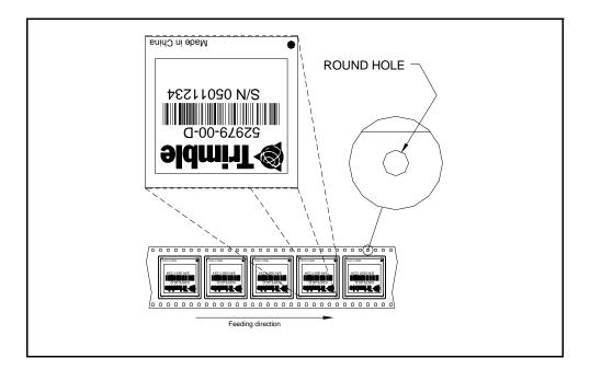
Figure 8.4 Feeding Direction Diagram
