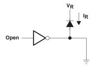
Figure 6. I<sub>R</sub> Test Circuit
