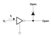
Figure 3. I<sub>I(on)</sub> Test Circuit
