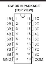
Applications include relay drivers, hammer drivers, lamp drivers, display drivers (LED and gas discharge), line drivers, and logic buffers. The ULN2803A has a 2.7-k $\Omega$  series base resistor for each Darlington pair for operation directly with TTL or 5-V CMOS devices.
