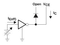
Figure 2. I<sub>I(off)</sub> Test Circuit
