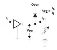
Figure 5.  $h_{FE}$ ,  $V_{CE(sat)}$  Test Circuit
