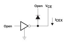
Figure 1. I<sub>CEX</sub> Test Circuit
