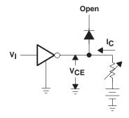
Figure 4. V<sub>I(on)</sub> Test Circuit
