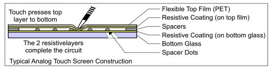
The 2 sheets are coated with a resistive substance, usually a metal compound called Indium Tin Oxide (ITO). The ITO is thinly and uniformly sputtered onto both the glass and the PET layer. Tiny bumps called spacer dots are then added to the glass side, on top of the resistive ITO coating, to keep the PET film from sagging, causing an accidental or false touch.
