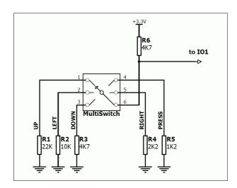
Unused buttons do not need resistors to be connected to the circuit. Table below lists the buttons and corresponding resistor values.
