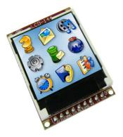
The **uLCD-144(GFX)** is a compact and cost effective display module using the latest state of the art LCD (TFT) technology with an embedded GOLDELOX-GFX2 graphics processor that delivers 'standalone' functionality to any project.
