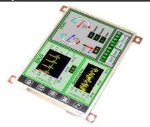
The uLCD-32PT(GFX) is a compact and cost effective all in one 'SMART" display module using the latest state of the art LCD (TFT) technology with an embedded PICASO-GFX2 graphics controller that delivers 'stand-alone' functionality to any project.
