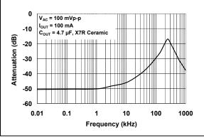
FIGURE 2-12: Power Supply Ripple Rejection (PSRR).
