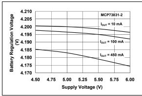
**FIGURE 2-1:** Battery Regulation Voltage (V<sub>BAT</sub>) vs. Supply Voltage (V<sub>DD</sub>).
