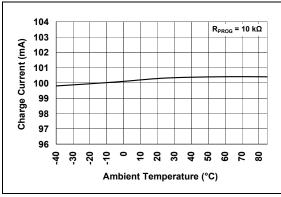
**FIGURE 2-7:** Charge Current  $(I_{OUT})$  vs. Ambient Temperature  $(T_A)$ .
