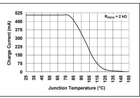
**FIGURE 2-10:** Charge Current  $(I_{OUT})$  vs. Junction Temperature  $(T_J)$ .
