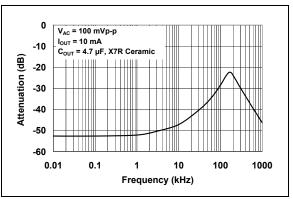
FIGURE 2-11: Power Supply Ripple Rejection (PSRR).
