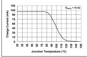
**FIGURE 2-9:** Charge Current ( $I_{OUT}$ ) vs. Junction Temperature ( $T_J$ ).
