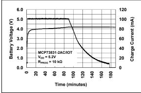
FIGURE 6-2: Typical Charge Profile (180 mAh Battery).
