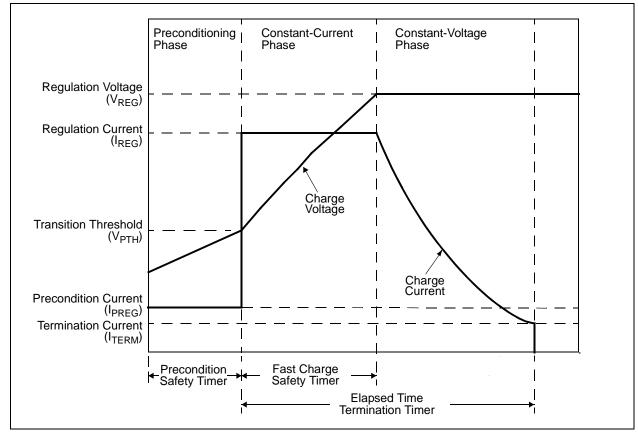
FIGURE 6-2: Typical Charge Profile.
