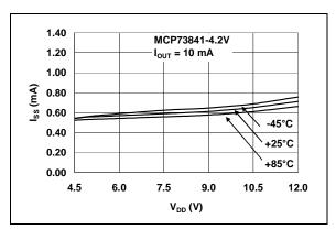
**FIGURE 2-6:** Supply Current ( $I_{SS}$ ) vs. Supply Voltage ( $V_{DD}$ ).
