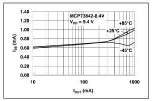
**FIGURE 2-10:** Supply Current ( $I_{SS}$ ) vs. Charge Current ( $I_{OUT}$ ).
