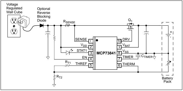
FIGURE 6-1: Typical Application Circuit.
