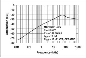
**FIGURE 2-21:** Power Supply Ripple Rejection.
