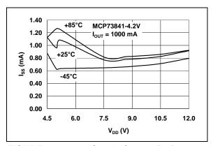
**FIGURE 2-5:** Supply Current ( $I_{SS}$ ) vs. Supply Voltage ( $V_{DD}$ ).
