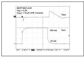
FIGURE 2-20: Load Transient Response.
