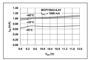
**FIGURE 2-11:** Supply Current ( $I_{SS}$ ) vs. Supply Voltage ( $V_{DD}$ ).
