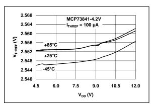
**FIGURE 2-15:** Thermistor Reference Voltage ( $V_{THREF}$ ) vs. Supply Voltage ( $V_{DD}$ ).
