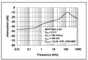
**FIGURE 2-24:** Power Supply Ripple Rejection.
