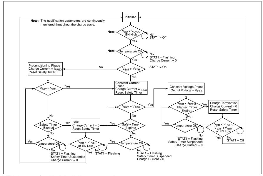
FIGURE 4-1: Operational Flow Algorithm - MCP73841 and MCP73842.
