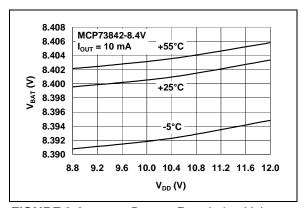
**FIGURE 2-9:** Battery Regulation Voltage  $(V_{BAT})$  vs. Supply Voltage  $(V_{DD})$ .
