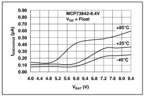
FIGURE 2-16: Output Reverse Leakage Current (I<sub>DISCHARGE</sub>) vs. Battery Voltage (V<sub>BAT</sub>).
