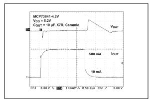
FIGURE 2-23: Load Transient Response.
