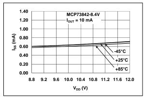
**FIGURE 2-12:** Supply Current ( $I_{SS}$ ) vs. Supply Voltage ( $V_{DD}$ ).
