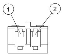
Connector B Manfacturer - JST Part #s PHR-2 Crimp Pin Part # SPH-002T-P0.5S Or equivalent Wire Entry View **Scale 5.00**
