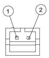
Connector A Manfacturer - JST Part #s S2B-PH-K-S Plug entry view
