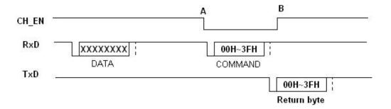
In Which: CH\_EN is an input signal to the wireless module.
