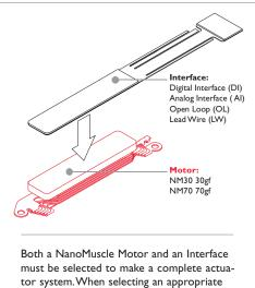
tor system. When selecting an appropriate actuator, please refer to the data sheets for both the NanoMuscle Motors and Interfaces.
