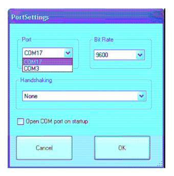
From device manager, we know that the COM port we are using is COM17. The default baud rate for PLC-UART is 9600. Click "OK", and Click "Open COM Port" to open the COM port.
