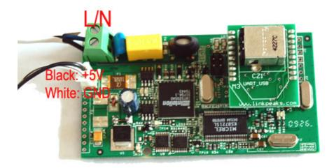
The AC or DC powerline line can be connected to the L/N connector denoted on the above picture.
