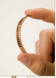
The Flex Sensor patented technology is based on resistive carbon elements. As a variable printed resistor, the Flex Sensor achieves great form-factor on a thin flexible substrate. When the substrate is bent, the sensor produces a resistance output correlated to the bend radius—the smaller the radius, the higher the resistance value.
