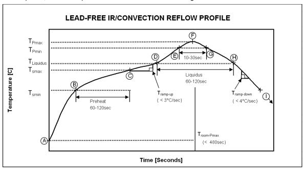
**Approved IR/Convection Solder Reflow Curve**
