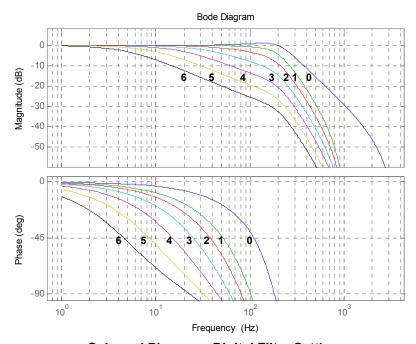
Gain and Phase vs. Digital Filter Setting
