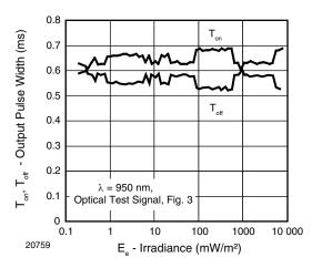
Fig. 4 - Output Pulse Diagram
