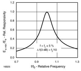
Fig. 5 - Frequency Dependence of Responsivity
