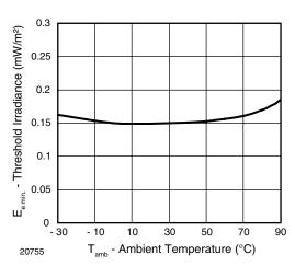
Fig. 10 - Sensitivity vs. Ambient Temperature
