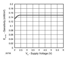
Fig. 14 - Sensitivity vs. Supply Voltage
