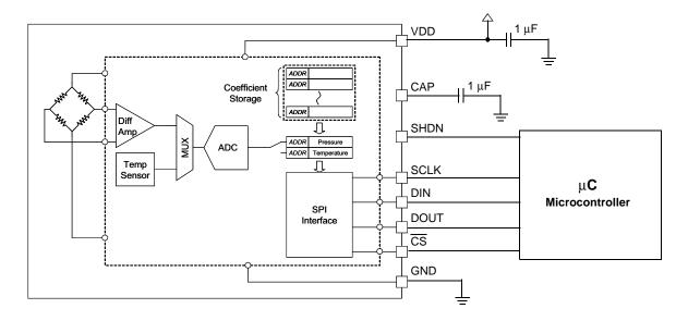
Figure 1. Uncompensated Pressure Sensor Schematic
