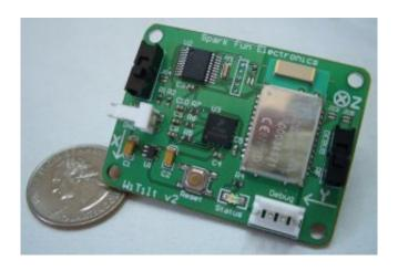
WiTilt v2 2.4GHz Wireless Dual-axis Tilt Sensor 10/12/2005
