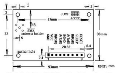
Sketch map of structural size of series HAC-LN wireless data-transceiver module
