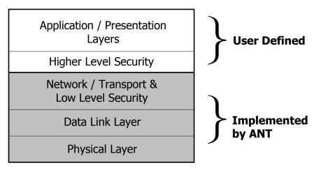
Figure 1-1: OSI Layer model of ANT
