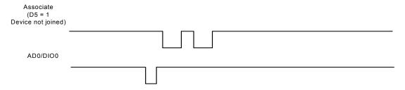
A single commissioning button press when the device has not joined a network that causes the associate pin to blink to indicate the AI Code where: AI = # blinks + 0x2 In this example, AI = 0x22.
