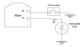
A pushbutton and an LED can be connected to module pins 20 and 15 respectively to support the commissioning pushbutton and associate LED functionalities.
