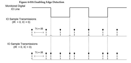
Enabling Edge Detection will force an immediate sample of all monitored digital IO lines if any digital IO lines change state.
