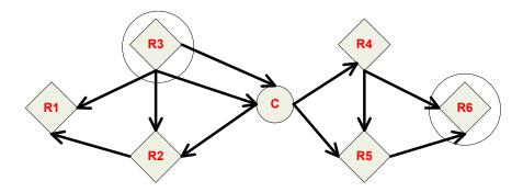
When the destination node receives a route request, it compares the 'path cost' field against previously received route request commands. If the path cost stored in the route request is better than any previously received, the destination node will transmit a route reply packet to the node that originated the route request. Intermediate nodes receive and forward the route reply packet to the source node (the node that originated route request).
