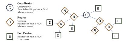
**Coordinator** – Responsible for selecting the channel and PAN ID. The coordinator starts a new PAN. Once it has started a PAN, the coordinator can allow routers and end devices to join the PAN. The coordinator can transmit and receive RF data transmissions, and it can assist in routing data through the mesh network. Coordinators are not intended to be battery-powered devices. Since the coordinator must be able to allow joins and/or route data, it should be mains powered.
