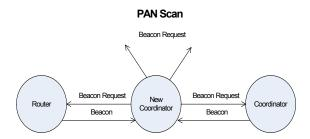
A PAN Scan allows the coordinator to detect nearby PAN IDs to avoid duplicating existing PAN IDs
