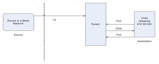
When RF data is sent to a sleeping end device, the end device's parents buffers the data until the end device polls for the data, or a timeout occurs
