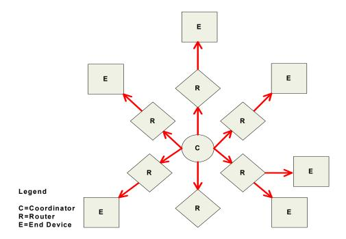
Each node that transmits the broadcast will also create an entry in a local broadcast transmission table. This entry is used to keep track of each received broadcast packet to ensure the packets are
