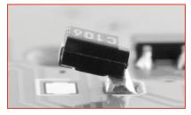
This is how a tantalum capacitor should look after making both solder connections.
