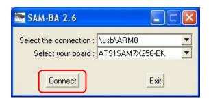
Select the USB connection and locate your board from the list of Atmel boards. Click "Connect" to start the Atmel SAM-BA utility.
