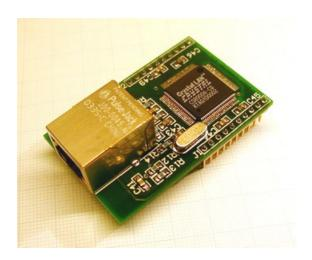
The IET8900 is a small form factor Ethernet access module. The module will allow almost any embedded system to connect to a 10Base-T Ethernet network. While this module was designed to accommodate the needs for test systems and DIY projects it is also very well adapted for small volume production runs where Ethernet connectivity is an option for the end user.
