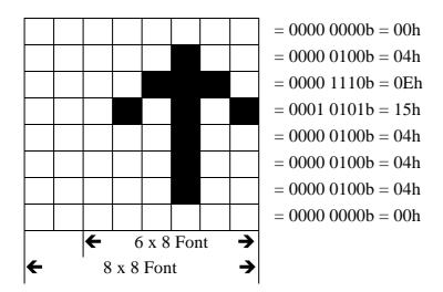
Assuming the CG RAM area is set to 1800 - 1FFFh, set the address pointer to location 1C00h (1800h + 80h x 8) as per section 5.5.1, and write the above 8 bytes using "write then increase" (section 5.5.2) or "data auto write" (section 5.5.4). Then setting the address pointer to an address in the text area, and writing '80h' will display the  $\uparrow$  character.
