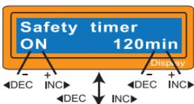
When you start a charge process, the integral safety timer automatically starts running at the same time. This is programmed to prevent overcharge the battery if it proves to be faulty, or if the termination circuit cannot detect the battery full. The value for the safety timer should be generous enough to allow a full charge of the battery .
