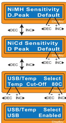
This shows the trigger voltage for automatic charge termination of NiMH and NiCd battery. The effective value ranges from 5 to 20mV per cell .if the trigger voltage is set higher, there is a danger of overcharging the battery; if it is set lower, there is a possibility of premature termination. Please refer the technical specification of the battery.(NiCd default:12mV, NiMH default:7mV)
