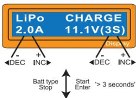
The left side of the first line shows the type of battery you select at the users setting. The value on the left side of second line sets a charge current and the value on the right side of second line sets the voltage of the battery pack.
