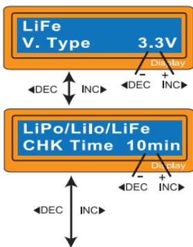
The screen displays the nominal voltage of Lithium battery. There are three kinds of Lithium battery; LiFe(3.3V),LiIo(3.6V) or LiPo(3.7V). This is very important so you have to check the battery carefully and set it up correctly. If it is different from correct value the battery can explode during charge process.
