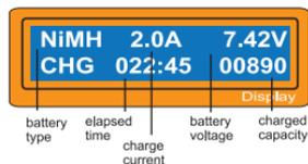
The screen displays the current state of charging . To stop the process, press Batt type/Stop key once.
