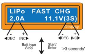
You can set up the charging current and the voltage of the battery pack being charged. As you press Start/ Enter button the voltage confirmation will be displayed. And then, if you confirm the voltage and current, press Start/ Enter button again to start charging.
