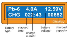
The screen displays the state of charging process. To stop charging forcibly, press Batt type/Stop key once.
