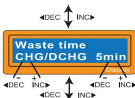
The battery is on the cyclic process of charge and discharge can often become warm after charge or discharge period. The program can insert a time delay to occur after each charge and discharge process to allow the battery adequate time to cool down before being subjected to the next process. The value ranges from 1 to 60 minutes.
