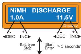
Set discharge current on the left and final voltage on the right. The discharge current ranges from 0.1 to 1.0A and the final voltage ranges from 0.1 to 25.0V). To start the process, press Start /Enter key more than 3 seconds
