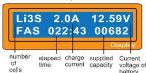
This shows the present state of 'FAST'charging. To stop charging arbitrary, press Batt type/ Stop key once.
