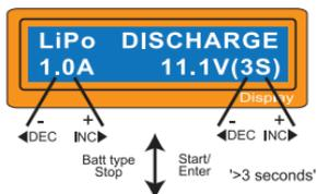
The value of discharge current on the left side of screen may not exceed 1C for a maximum safety and the final voltage on the right should not be under the voltage level that is recommended by the battery manufacturer to avoid deep discharging.
