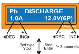
Set discharge current on the left and final voltage on the right. The discharge current ranges from 0.1 to 1.0A.
