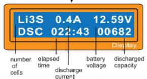
This shows the present state of discharge. To stop discharging press Batt type/Stop key once.
