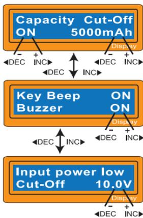
This program sets the maximum charge capacity that will be supplied to the battery during charge. If the delta-pack voltage is not detected nor the safety timer expired by any reason, this feature will automatically stop the process at the selected capacity value.
