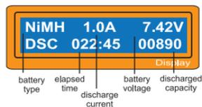
The screen displays the current state of discharge. You can alter the discharge current by pressing Start/Enter key during the process. Once you change the current value, store it by pressing Start /Enter button again.
