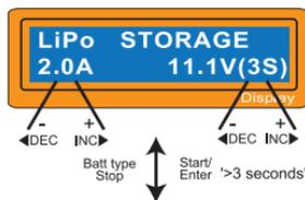
You can set up the current and the voltage of the battery pack to be charged. The current will be used for charge or discharge the battery to reach the 'storage' level of voltage.
