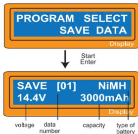
The parameter value setting up in this screen does not affect charge or discharge process. They only represent the specification of the battery. The following screens will automatically be displayed exactly matched with the
