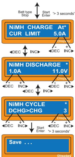
battery type you set up. The example shows the battery pack of NiMH, 12cells and 3000mAh of capacity.
