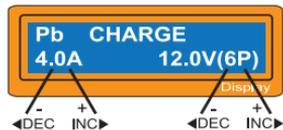
Set up the charge current on the left and the nominal voltage of the battery on the right. The charge current ranges from 0.1 to 5.0A and the
