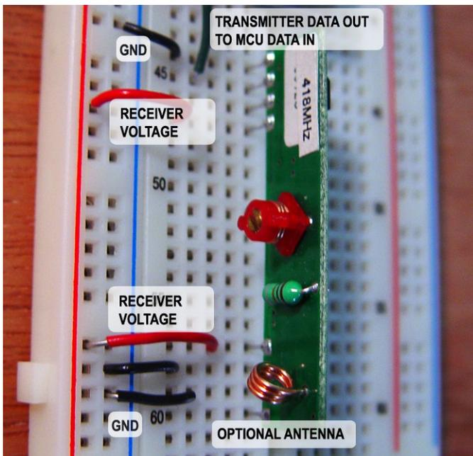
The receiver modules all share common pin assignments, as follows (from the top). Pin 1 goes to ground. Pin 2 sends the incoming byte from the transmitter out to the microcontroller. Pin 3 needs no connection, but can be taken to ground. Pins 4 and 5 go to the receiver voltage. Pins 6 and 7 go to ground, leaving Pin 8 as the optional antenna pin. Quite simply, that's all there is to it!
