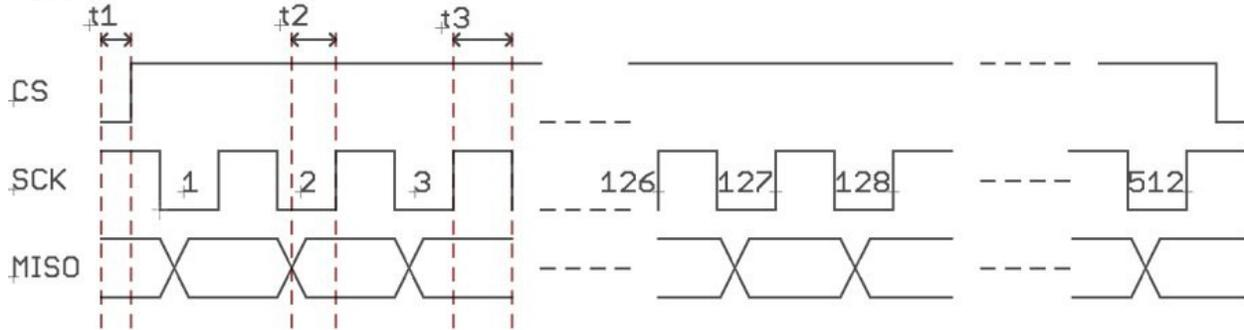
Figure 4 shows how the external device should control the signals to send a set of data (remember, a data set consists of 4 frames of data). Notice how the data on the MISO line is only changed while the SCK is low. This is also true for the MOSI line; which means if you are reading data from the Button Pad Controller SPI you should do so only while the SCK line is high. The data will not be valid while the SCK line is low.
