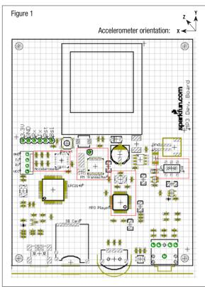
There are several key components worth discussing pertaining to the hardware layout. There is a programming header, along with a debug header; neither of which come populated on the board. Rather than using the programming header, the user should load new code to the SD card through the on-board USB port.
