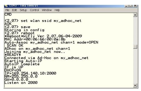
Alternatively you can statically set the IP address by disabling the DHCP service and explicitly assigning the IP address.
