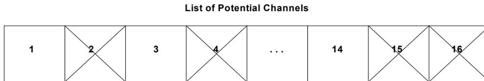
Performing an energy scan allows the coordinator to avoid starting on channels with high energy levels.
