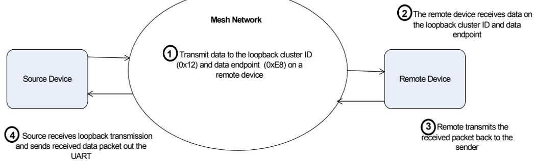
Demonstration of how the loopback cluster ID and data endpoint can be used to measure the link quality in a mesh network
