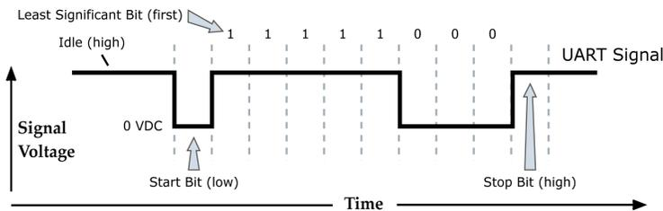
The module UART performs tasks, such as timing and parity checking, that are needed for data communications. Serial communications depend on the two UARTs to be configured with compatible settings (baud rate, parity, start bits, stop bits, data bits).
