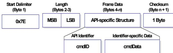
The cmdID frame (API-identifier) indicates which API messages will be contained in the cmdData frame (Identifier-specific data). Note that multi-byte values are sent big endian. The XBee ZNet 2.5 modules support the following API frames:
