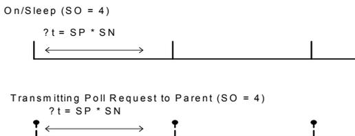
Setting SO = 4 will cause the end device to sleep for the entire SP \* SN time. This should only be used if the end device will not receive RF data while sleeping.
