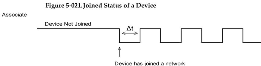
**The associate pin can indicate the joined status of a device . Once the device has joined a network, the associate pin toggles state at a regular interval ( $\Delta t$ ). The time can be set by using the LT command.**
