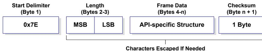
MSB = Most Significant Byte, LSB = Least Significant Byte
