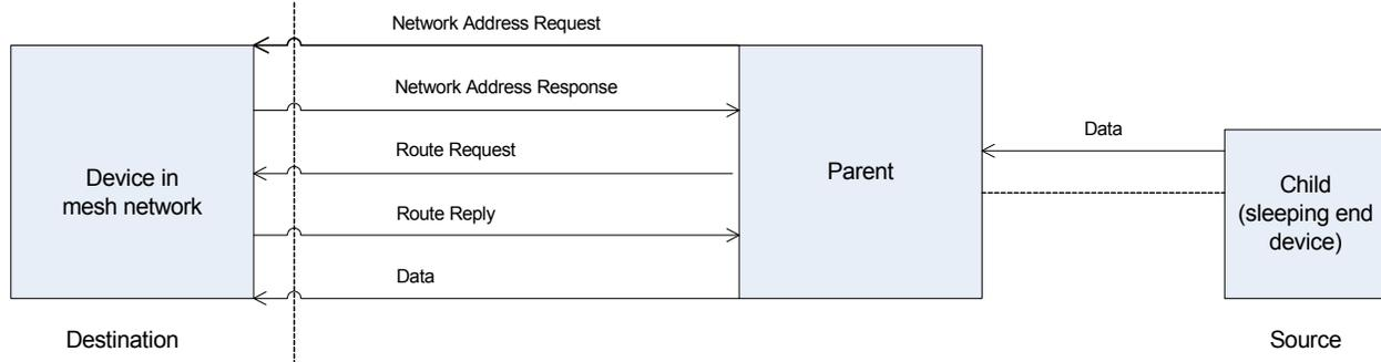
**An end device sends data to its parent to route to the correct destination node. The parent performs all of the necessary addressing and route discoveries before forwarding the data.**
