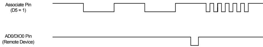
**A single button press on a remote device causes a broadcast node identification transmission to be sent. All devices that receive this transmission blink their associate pin rapidly for one second if the associate LED functionality is enabled. (D5 = 1)**
